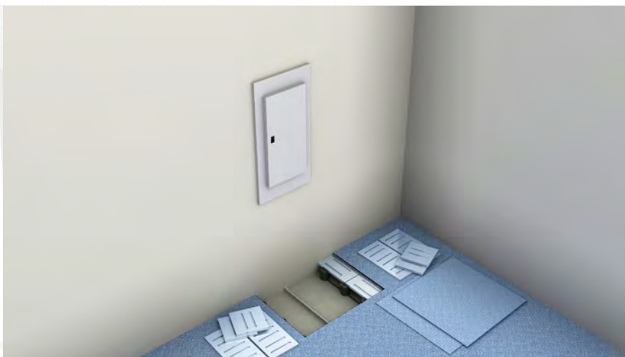
Homerun Cable to Electrical Panel - (3 circuits each)
